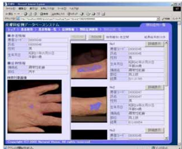
Figure 4 Screen capture of image database system. In this system, the user dermatologist specifies the region of interest (blue mark in the image), and image-based retrieval can be done by the spectral similarity of the specified regions.
