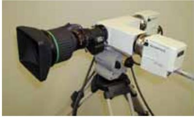
Fig.5 6-band HDTV camera
