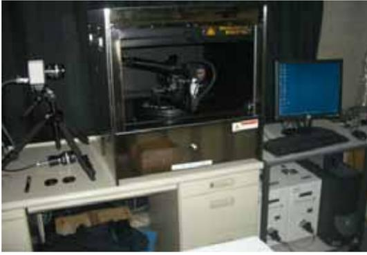
Fig.15 The multispectral BRDF/BTF measurement system.
