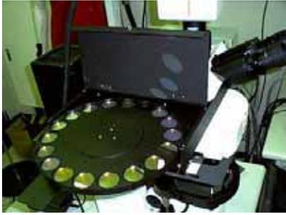
Fig.11 Filter wheel in the 16-band microscopic image acquisition system.
