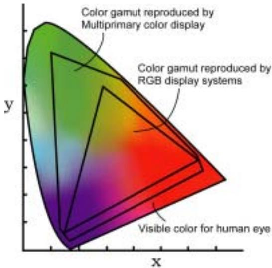
Fig.3 The concept of gamut expansion by multiprimary-color display
