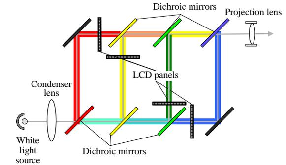
Fig.4 The examples of optical systems for multiprimary color projection display
