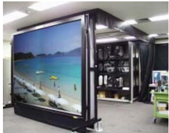
Fig.6 Six-primary 2x2 multi-projection display system with about 2300x2000 resolution
