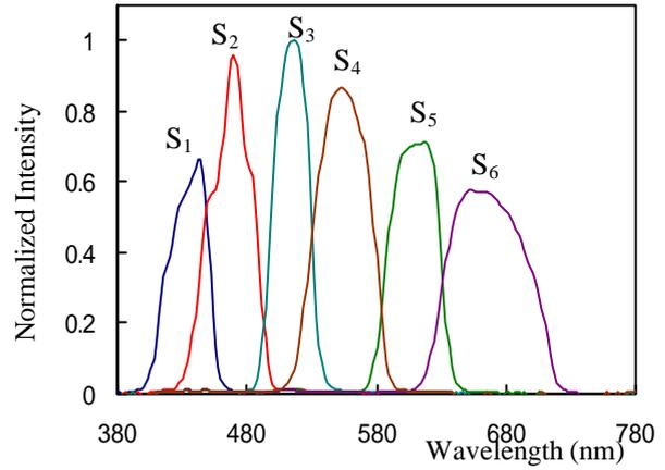
Fig.4 The spectral intensities of six-primary colors
