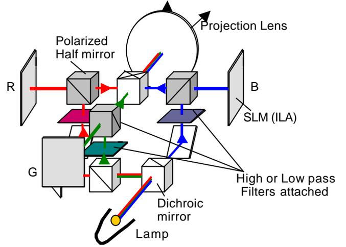
Fig.2 The optical setup for the six-primary projection display prototype (on the one projector's side).
