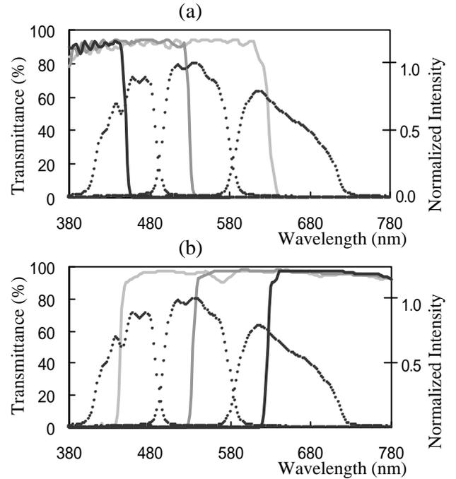
Fig.3 The spectral transmittances of (a) low-pass and (b) high-pass filters. The spectral intensities of RGB lights are also shown (dotted line), respectively.
