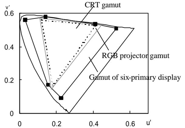
Fig.5 The color gamut by the six-primary projection system(solid line). The color gamut of the conventional EBU phosphor (dotted line), and projector display(gray line) also shown.
